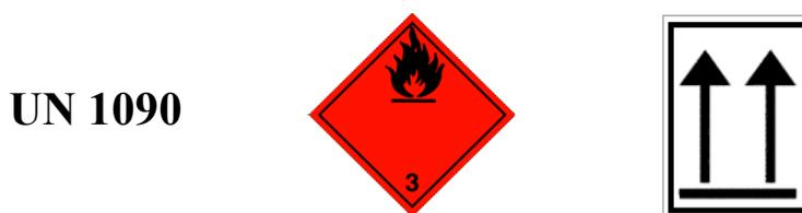
*Figure 1.* Examples of markings on a package. These goods contain a substance with UN number 1090 (acetone). The red label indicates that the substance is a flammable liquid. The flame indicates that the substance is flammable, while the number 3 indicates that the substance belongs to class 3, that is, flammable liquids. The arrows show which direction is up and which is down for the goods.
